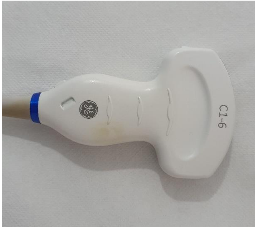
Figure 15: The curvilinear probe used for assessing liver characteristics during USG
